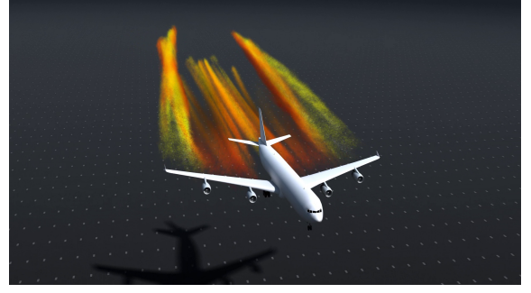
Figure 3: Large eddy simulation of the roll-up process for an A340 aircraft. Multiple vortices shed from the aircraft wings form a pair of two counter-rotating swirls.
